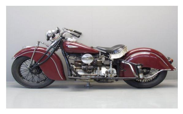
9. Indian, 1265cc Intake Over Exhaust (I.O.E.) In Line Four, 1927-42
