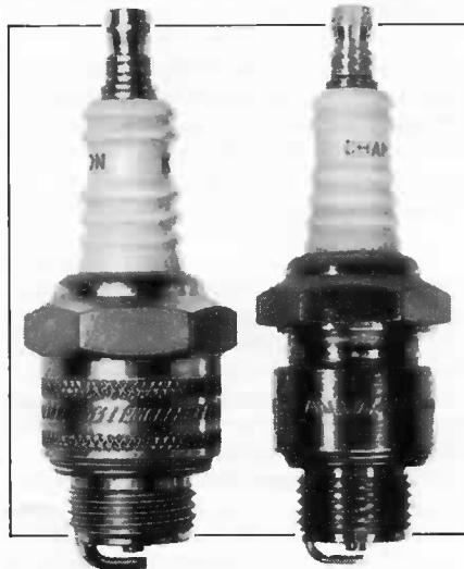
A pair of 18mm short reach plugs. On the left a cold one, on the right a hot.
