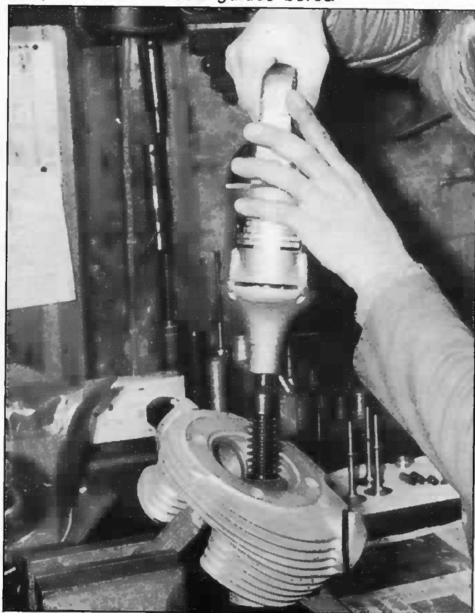
Steve Hayward carries out the final seat grinding operation on one of the many hundreds of Vincent heads processed by Maughan and Sons.
