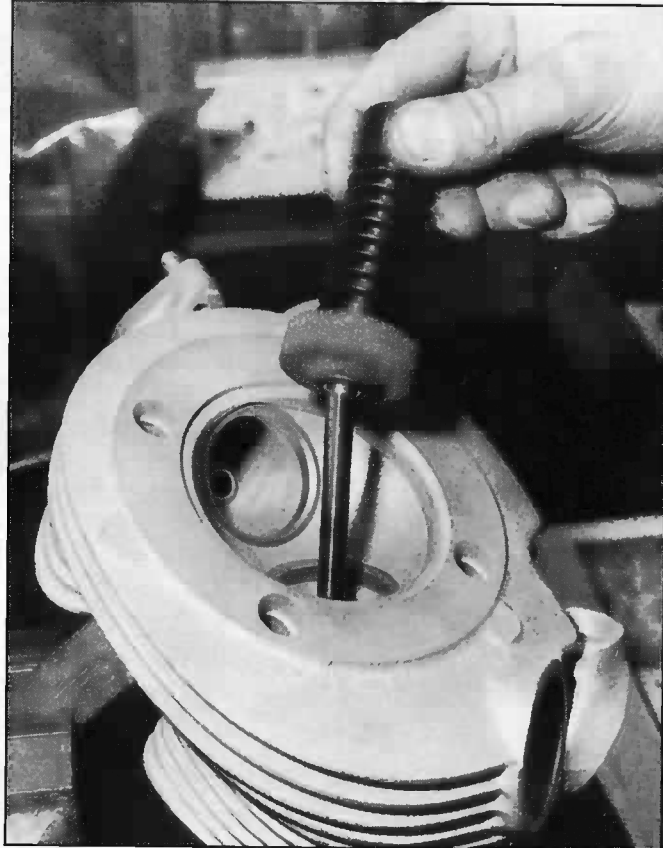
A hardened and ground piloting bar is locked into the lower guide. This bar is the central location for the grinding wheel which is used to generate the valve's seat, concentric to both guides' bores.
