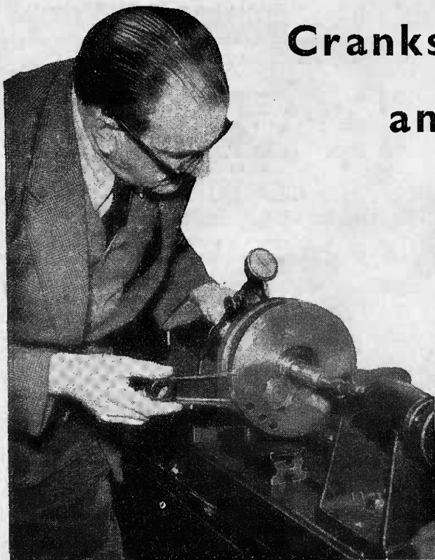
Mr. Hartley checks the run-out of a "Manx" Norton flywheel assembly. In this type of engine, readings are taken on the flywheel rims as well as on the mainshafts.
