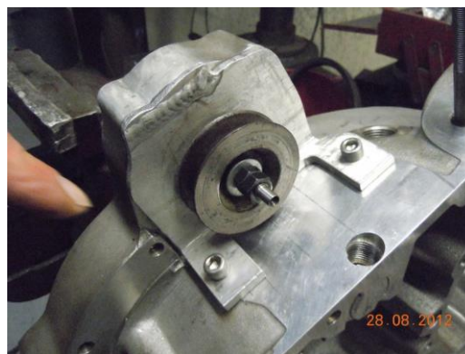
Bob McLennon & the generator jackshaft
