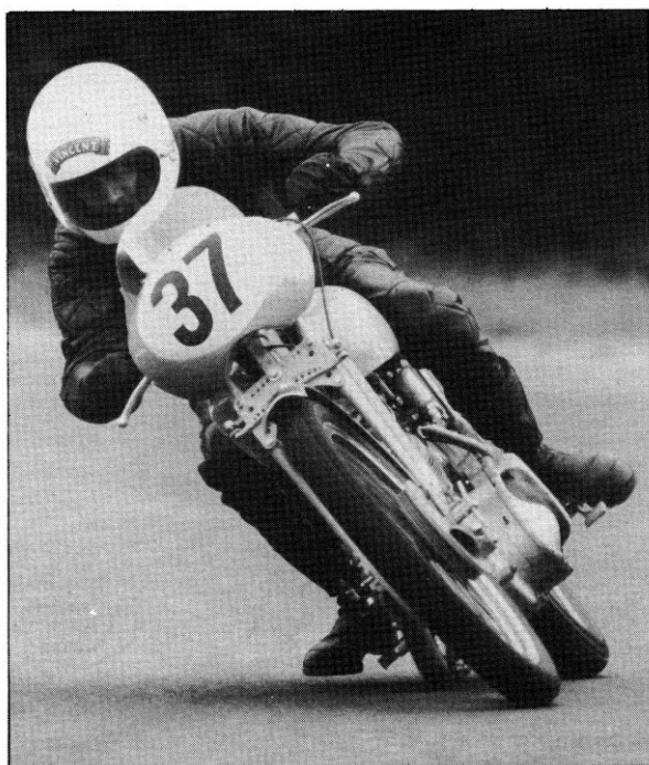
On the original restoration, the 2in exhaust pipe grounded too easily on right-handers
