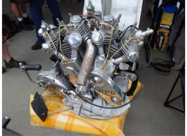
The C heads + barrels on an A lower end concept in the speedway motor was devised by K Carrick. 3 were made, Kal has 1 and Boyd has 2.
