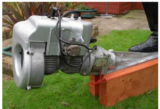
Next, I was introduced to the 200 c.c. sports version which is configured with 2 100 cc units bolted together to produce a parallel twin and is now just going into production: The extra cylinder volume increases the speed to some 8 to 10 m.p.h
