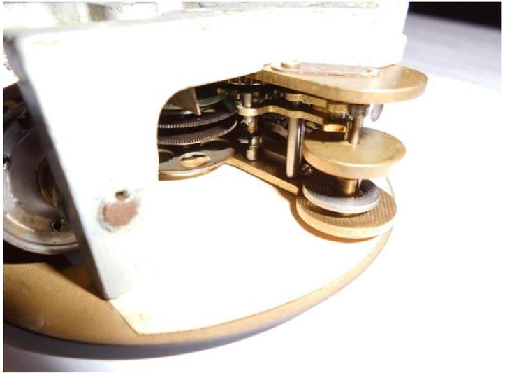
The stabilizer wheel has two functions. The first and lesser of these is to ensure an accurate zero position of the pointer. In the edge of the wheel a niche is cut, into which a small V shaped spring falls when the pointer returns to zero. In its more important function it is in effect an averaging device. There are 135 useful teeth on the edge of the integrator and recorder wheels, a factor which limits the accuracy to one part
