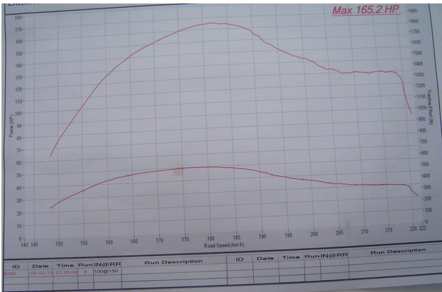
Rear wheel Dyno result from the new Terry Prince race motor
