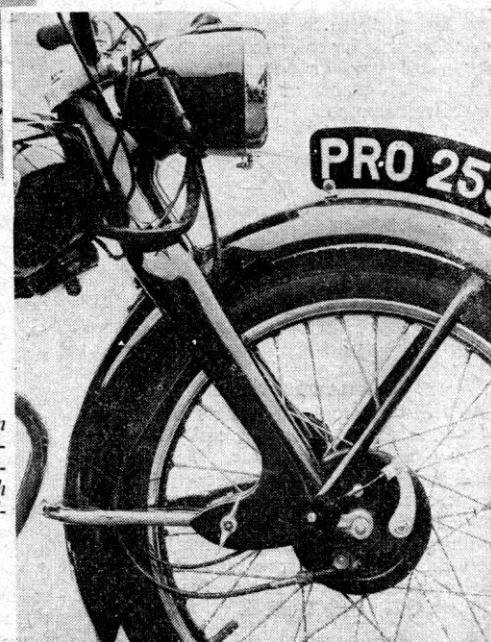
Of unusual design is the swinging-fork front suspension (right) which utilizes pressed-steel fork legs.
