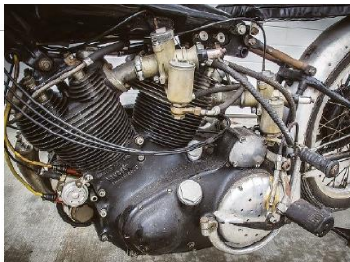
As found: Dehydrator plugs were screwed into the spark plug threads and inserted into corks in the carburetors.
