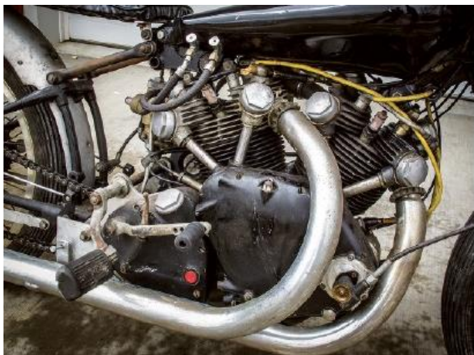
As found: Dehydrator plugs were screwed into the spark plug threads and inserted into corks in the carburetors.
