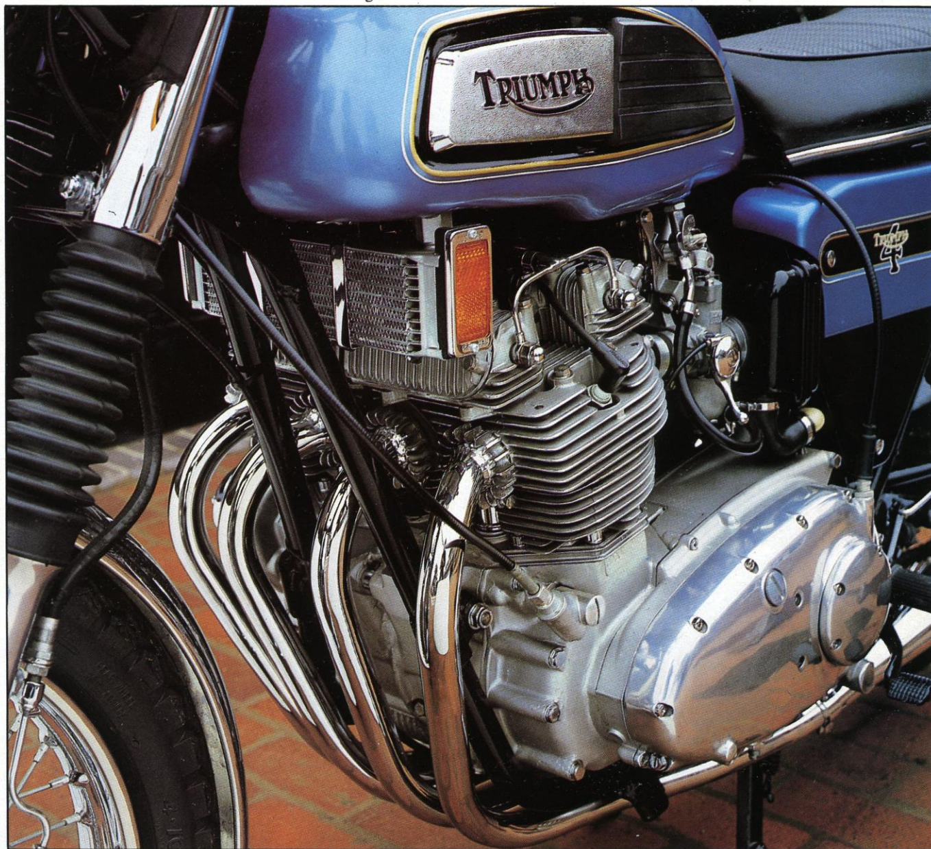
The Quadrant's cylinder block was formed from two Trident blocks, each with a cylinder removed. A production machine would have had block and head cast as one piece.
