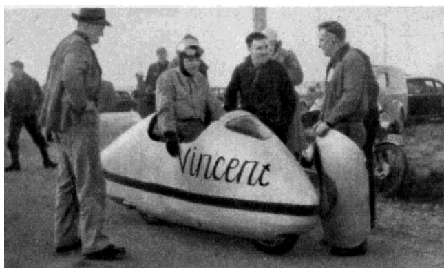
Two pictures of Robert Burns, of Christchurch, New Zealand, with the streamlined 998 c.c. Vincent "Rapide" outfit on which he set up a new British Empire sidecar record last month. Note (left) the hatch which completes the windcheating "egg."
