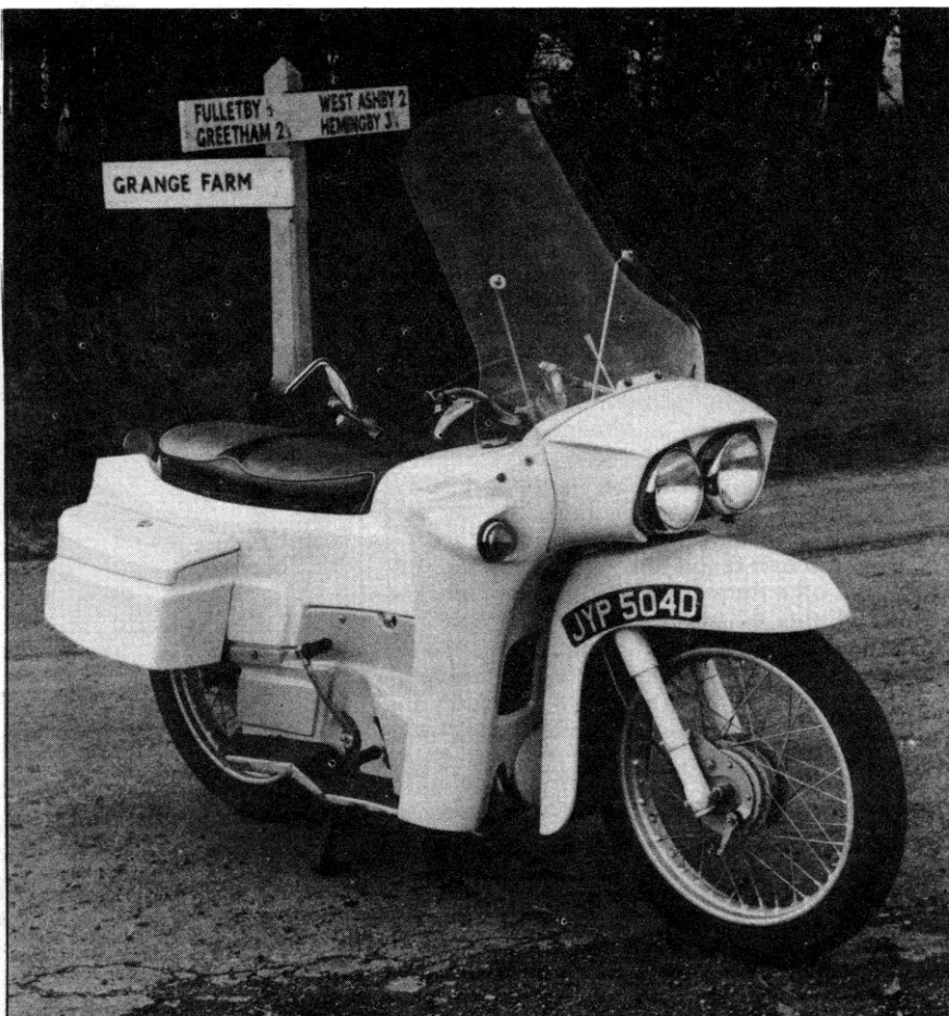
Fibreglass enclosure, twin headlights and faired-in indicators make the Velocette Vogue one of the most adventurous British designs of the sixties
