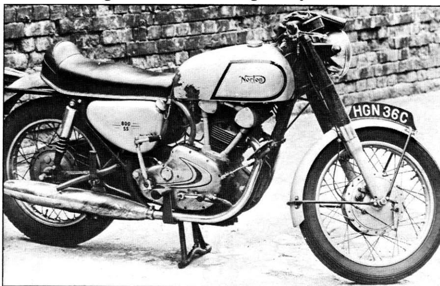
Looking like a tubby Vincent Comet, the 800cc dohc P10 was the twin the Commando replaced. The 'pushrod tubes' conceal the chain drive to the camshafts.
