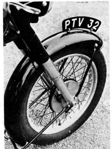
Below right: Front brake was inadequate. Note rear guard stay which doubles as a front wheel stand.
