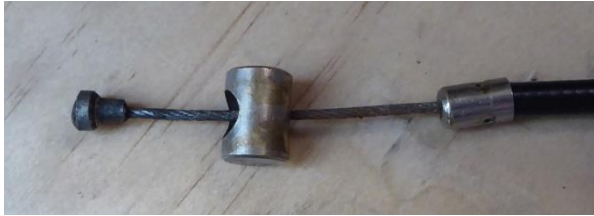
Lever end showing loose BN1013
