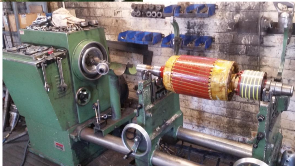
Photo Three: An overview of the 1950's Repco Dynamic Balancing machine in use, balancing an armature – and before anyone asks – no it's NOT from a Lucas magneto!
