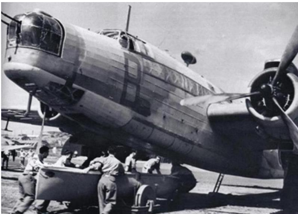
Crew fitting an aluminum lifeboat under a bomber. The purpose was for the bomber to drop the lifeboat to surviving air crew at sea so they could sail themselves to safety.
