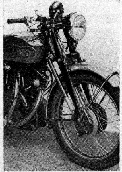
Extreme lateral rigidity is a feature of the massively - proportioned Girdraulic fork. The trail can be altered for sidecar work in a few minutes
