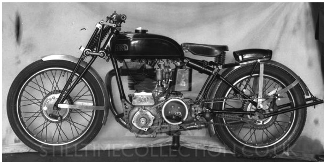
1934 HRD fitted with the revised 1934 JAP engine and a Burman gearbox
