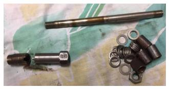
I located a piece of 3/8" bar that was threaded both ends and packed it up with spacers and washers then tightened it down into the insert and fitted it with a nut to firm everything up.
