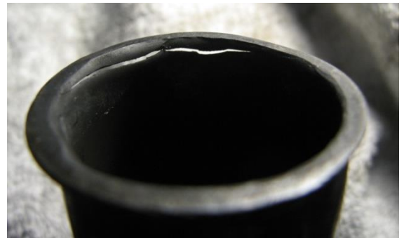
Pic showing exhaust with crack
