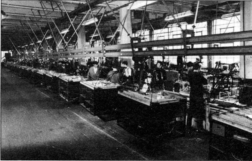
Automated assembly of singles and twins at Small Heath in the mid-sixties
