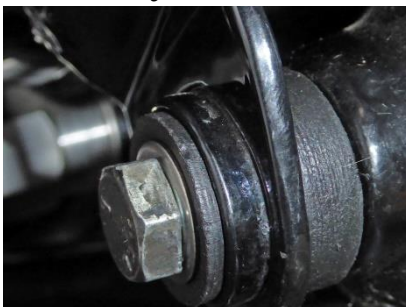
Done: FT80 no longer crushed and anti-vibration restored
