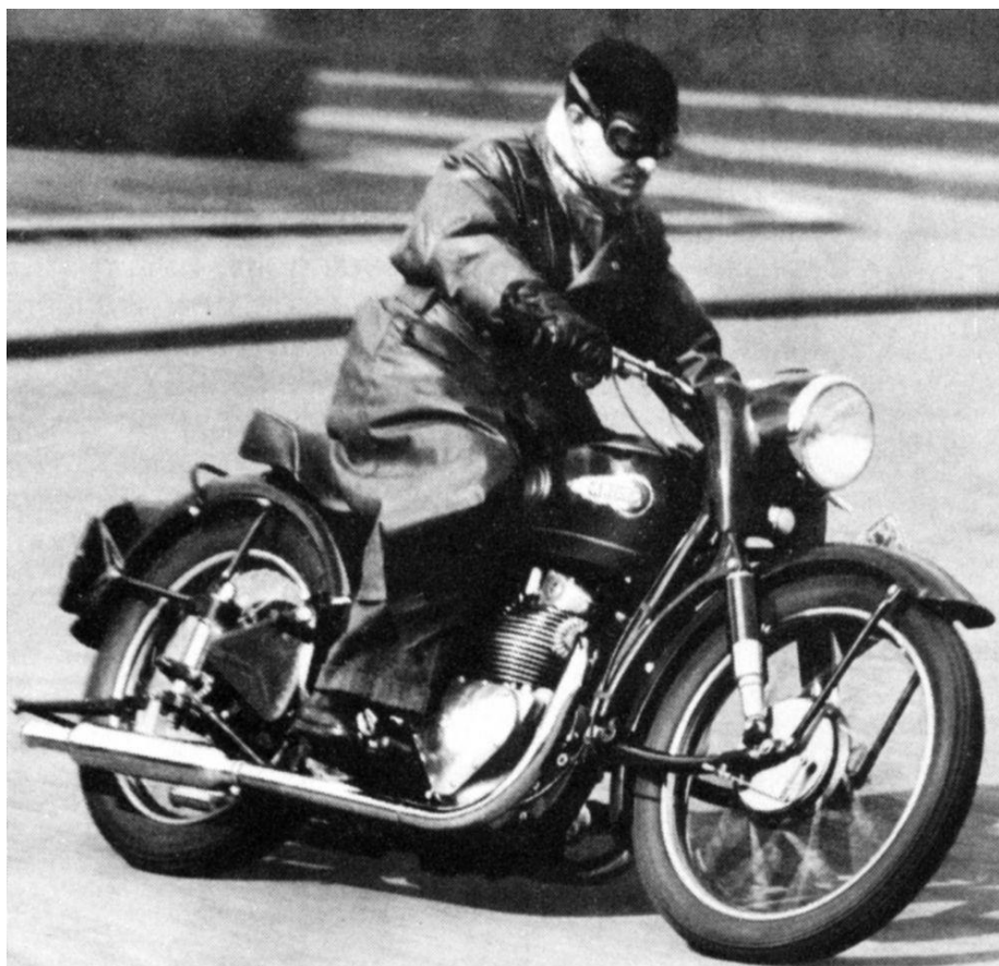
Prototype Ariel KHA Mk II Hunt Master twin on test. Unstable and considered by some as ugly
