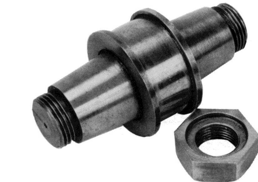
A tapered crankpin with rebated nut
