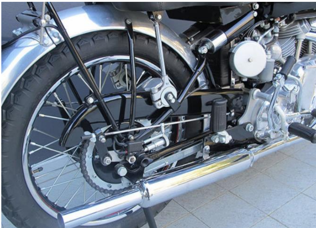
Standard Vincent rear suspension, with the seat firmly attached to the swing arm
