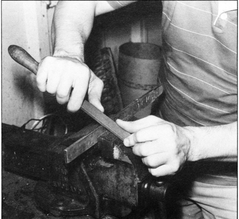
Draw filing is an ideal method for removing sharp edges. It also allows excellent file control when filing narrow surfaces.
