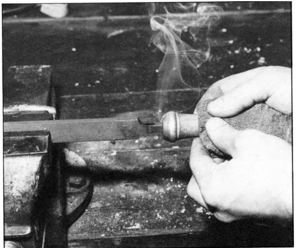
Correct fitting of the file's handle is essential. The tang should be burned into the handle prior to final fitting.
