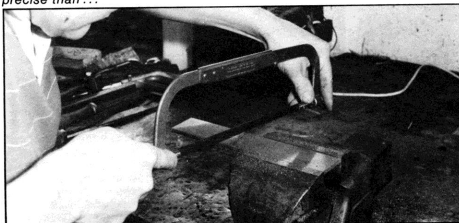
... cutting this way which has more teeth in contact with the work and is a more accurate method.
