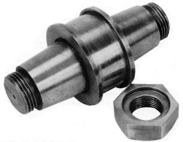
A tapered crankpin with rebated nut
