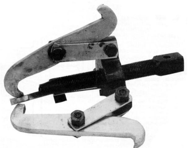
Pullers will remove sprockets and gears from taper joints
