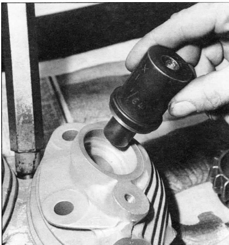
Special hard reamer steady bushings are clamped into the upper valve guide location prior to reaming the lower guide housing.
