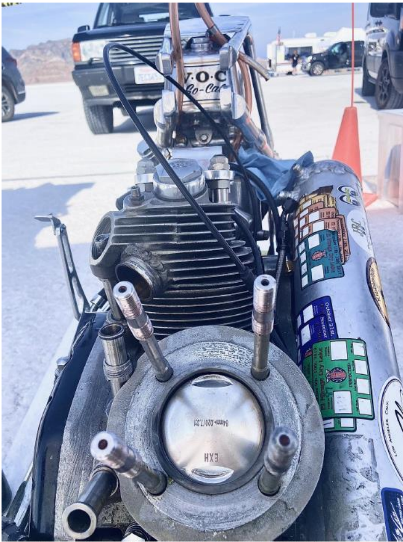
Figure 3 shows the stock 7.3:1 piston (stamped on the piston) during the tear-down. James Salter photo.
