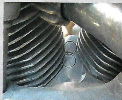
Crankcase halves are numbered in pairs. Look here on a Rapide
