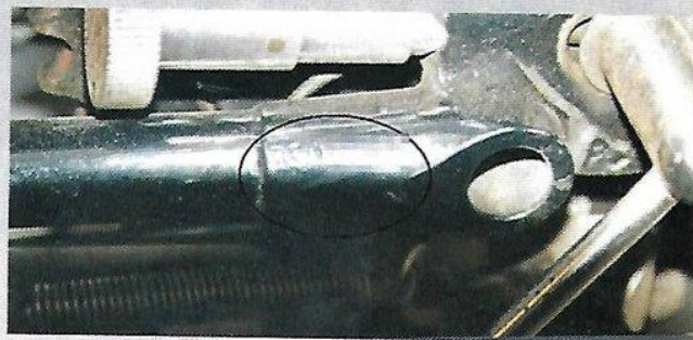
Rear frames are stamped here. The VOC can tell you which engines and frames were originally assembled by the factory. Great chain adjuster, too
