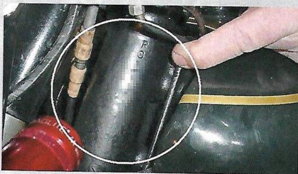
Front (or 'upper') frame numbers can be found here
