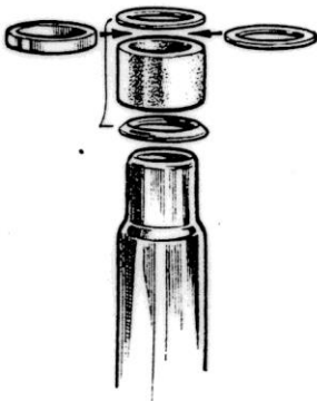
Packing rings of alternative thicknesses at the top of each push-rod tube compensate for removal or insertion of compression plates.
