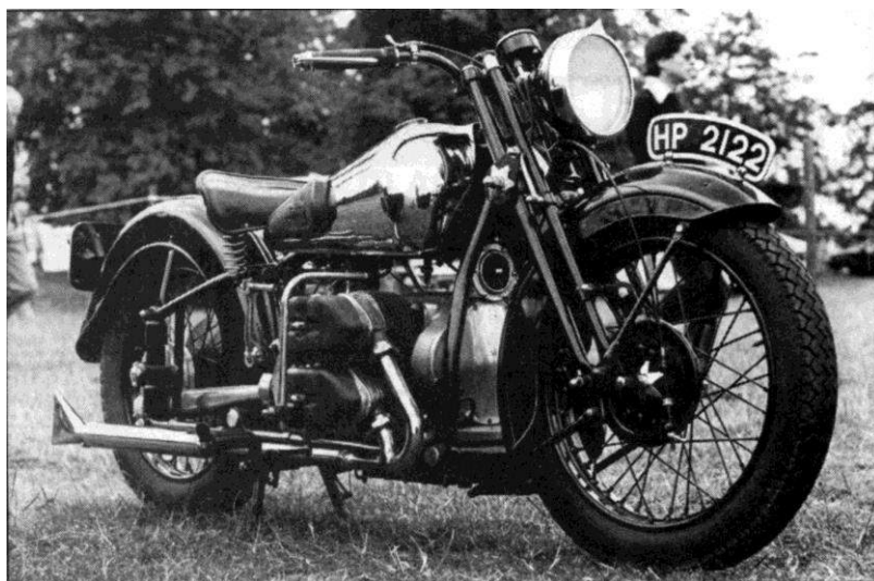
Brough as innovator: the flat-four Dream of 1938. Many factory models before it carried the HP 2122 plate
