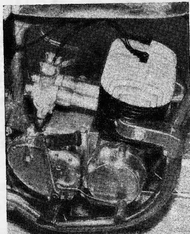
More uniform temperature distribution is the object of the side-mounted exhausts of the R.C.A. twin two-stroke.
