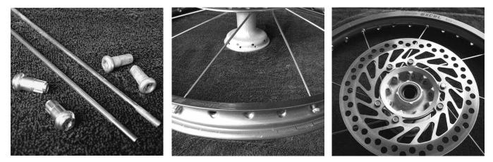
Left: The new pieces, left, are visibly more substantial than the stockers they replace. (Don't be fooled by the narrower threaded section on the Excel spoke; its shaft is thicker than OEM.) Right: The first row of new spokes, with nipples loosely attached. Right: Notice the even spacing along the rim.
