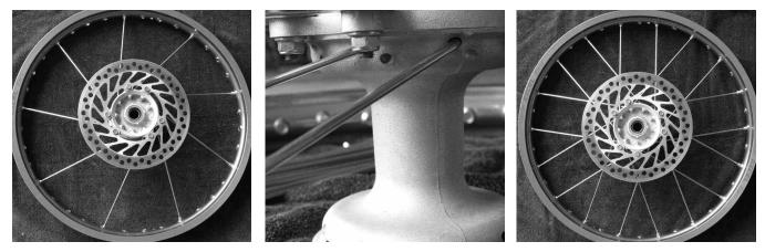
Left: One row of spokes finished. The wheel begins to take shape. Center: Detail of the spokes leaving the hub. Notice how the holes point only partway toward the spoke's target on the rim; the spoke's bend (right at the hole's edge) completes the necessary angle. Right: Halfway done; here's the wheel with one side (flange) of the hub laced.
