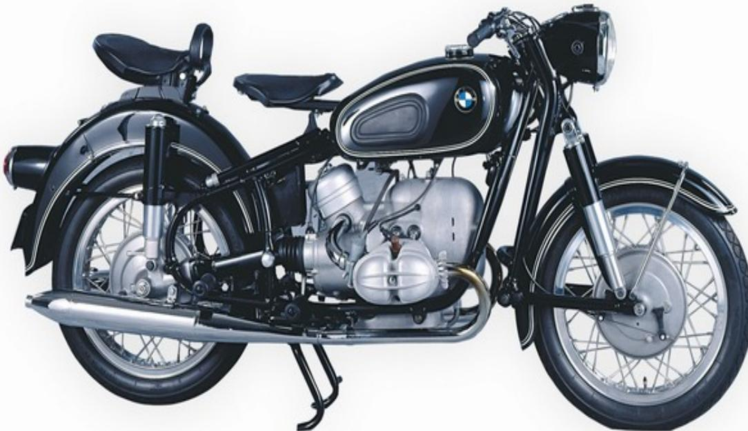
19. B.M.W. R69, 600cc "Boxer" Twin Horizontal Opposed Pushrod Operated O.H.V. 1958-9
