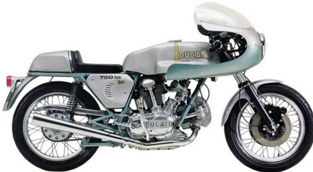
11. Ducati, 750cc Desmo SS Vee Twin, Shaft and Bevel Gear Driven O.H.C., 1974
