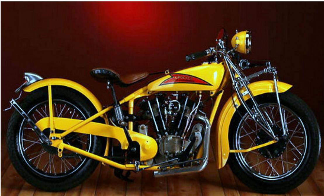
4. Crocker, Vee Twin 61 cubic inch O.H.V. Pushrod Operated, 1936-42
