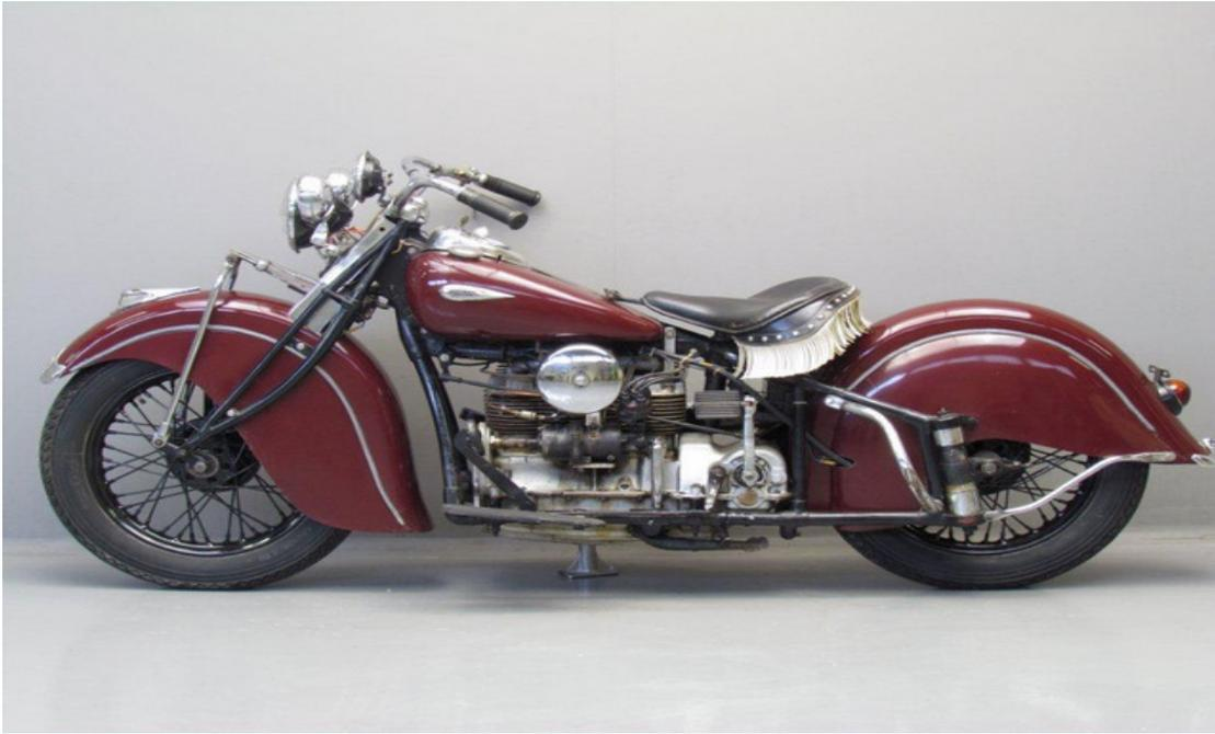
9. Indian, 1265cc Intake Over Exhaust (I.O.E.) In Line Four, 1927-42
