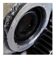
Here is the new seal, left from outside the crankcase, and right, from the timing chest side.
