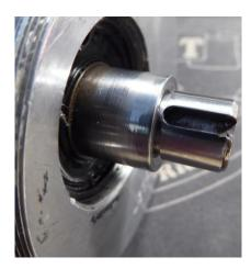
Here is a picture of the drive end of my Alton. Look carefully and you will note the diameter of the drive shaft is largest where it exits the alternator body and it is then reduced in diameter to accommodate the drive gear. This photo was taken after I had polished the larger diameter part of drive shaft (done without disassembly of the ALTON) ensuring the lipped seal had a smooth sealing surface.
