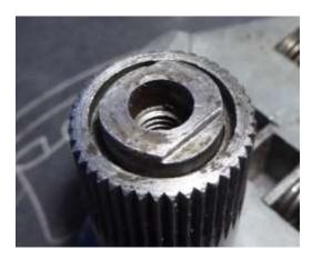
In OVR #36 Bernhard Kurschel described how to effectively fit an internal oil seal to the gear change shaft carrier. While this tamed at least 80% of the oil leaking from the gear change area, some traces of oil was still able to find its way to the outside world along the tiny space between PR50-C-094 the ratchet foot change sleeve and the inner PR50-C-090 sector spindle.
