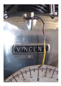
You need a pointer, a fixed position relative to the timing disk. I made mine from a length of soft wire (an old wire coat hanger) bent to shape. I painted the end just to make it easier to see.
