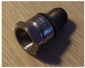
Here is a photo of my finished piston stop. Note that the nut is of a size that can pass thru the spark plug hole.
