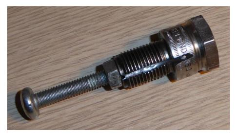
In use the piston stop is screwed into the spark plug hole but as you will be slowly turning the motor over by hand you want as little resistance as possible so you need to cut a channel into the side of the stop to allow compression gases/air to escape as you turn the motor over. I used a Dremel with a thin cutting disk to cut the channel in my piston stop.
