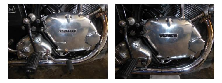
This is an opportune time to also remove the cap over the inlet valve adjuster and also the spark plug (with a twin, remove both spark plugs). The cap is removed so you can observe the movement of the inlet rocker as the motor is rotated; the spark plugs are removed so you are not 'fighting' against the compression pressure.
