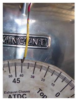
In my case the pointer was at 80 degrees when the piston made contact with the stop, so the mid-point to TDC on the DISK is 40 degrees, which is actually TDC of the MOTOR.
