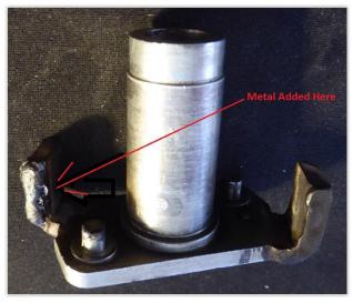
The photo, left, shows a fixed arm where metal has been added to the ears by welding. When doing this be sure to take precautions to avoid damaging the bob weight pivot pins. In retrospect it may have been better to add the metal to the faces of the 2 ears furthest from those pins.
