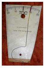
To find out what your ATD is presently doing you need to accurately measure the amount of advance it provides and it is not hard to do so. Make up a ATD Set Up Guide *Photo left is an example*; To make your own <u>CLICK HERE</u> to download a printable image. Print out the image (bigger is better) then glue it to some light plywood or like material, trim it to a convenient size and at the centre point drill a hole to take a snug fitting 3/8" BSF set screw or bolt.
