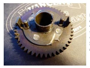
Some folks will tell you that the ATD range may by altered (or tuned) by BENDING the 'ears' on the ATD and while this is true it will create stress inside those bends that could lead to the ATD ears breaking off when in use. The ATD 'base' shown in Photo left had both its limit ears fail in use as a result of bending them when attempting to change the ATD range.
